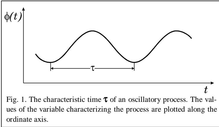
Fig. 1. The characteristic time  $\tau$  of an oscillatory process. The values of the variable characterizing the process are plotted along the ordinate axis.
